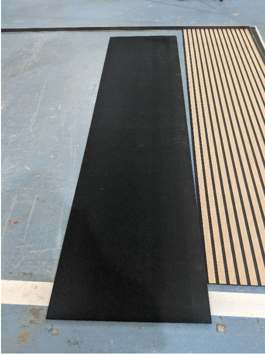
Figure 3 – Individual specimen panel, face oriented toward horizontal test surface
