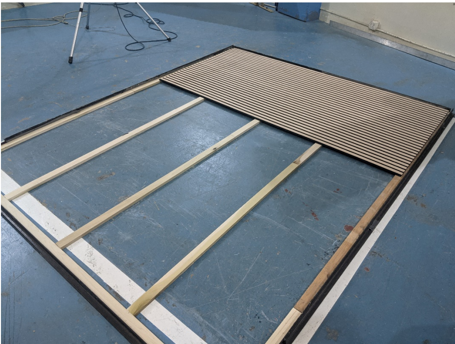
Figure 2 – Specimen partially installed over spaced furring strips
